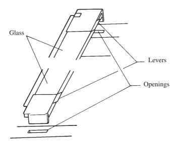
Figure 5.7 Inserting the glass
